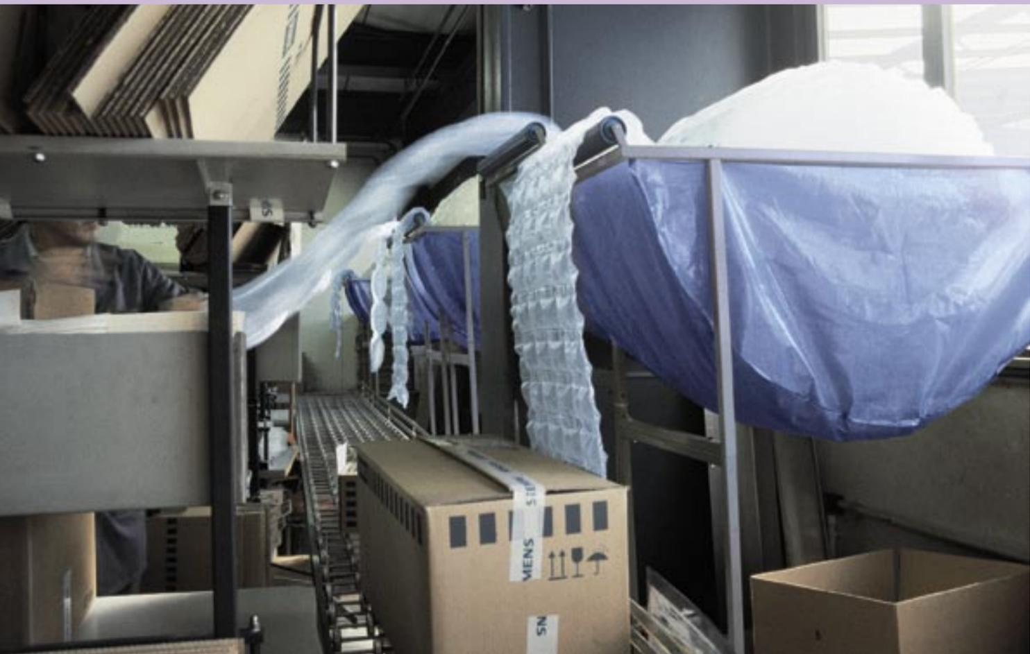
**The Airpad protection and void-filling material**
